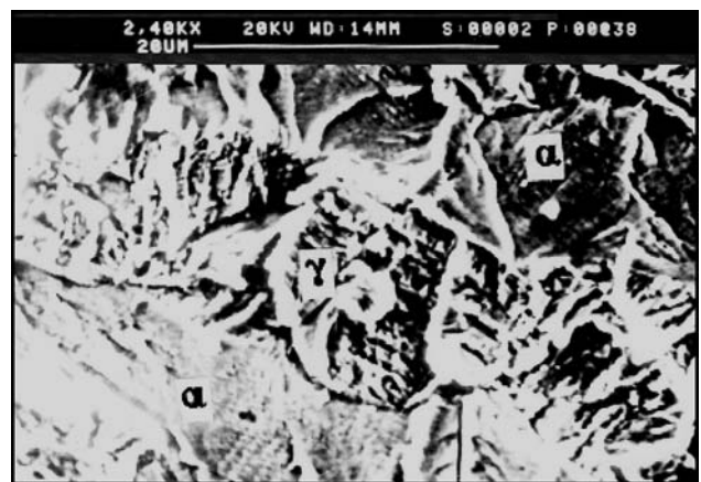
Fig. 9 Ductile tearing of austenite phase present in between ferrite cleavage facets
